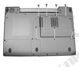
Figure 2-4 Remove the seven screws
